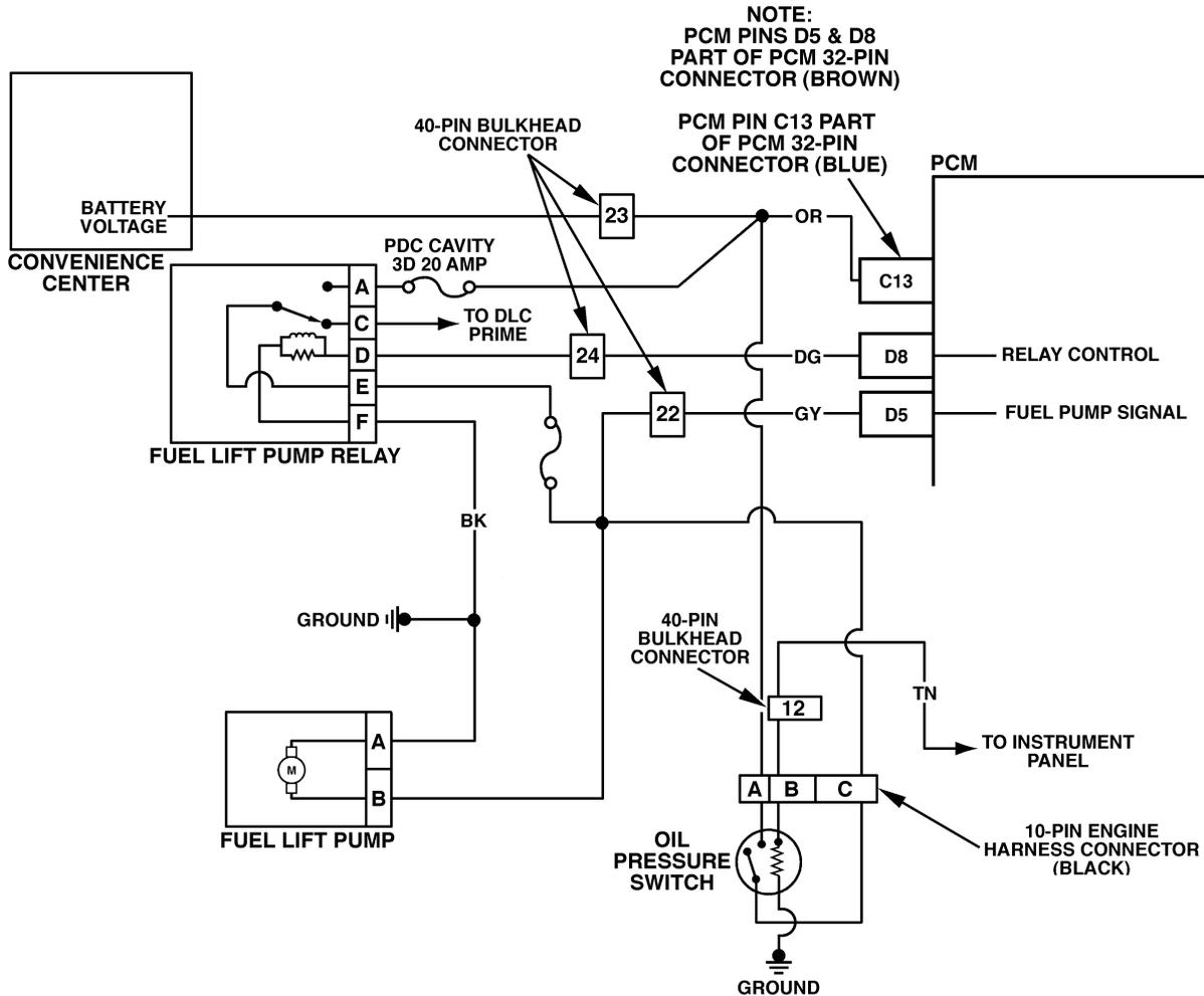
Figure PCM-22 Fuel Lift Pump Secondary Circuit Low Voltage
