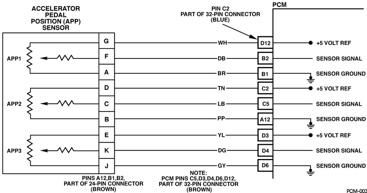
Figure PCM-15 Accelerator Pedal Position (APP) Sensor 2 Circuit Performance
