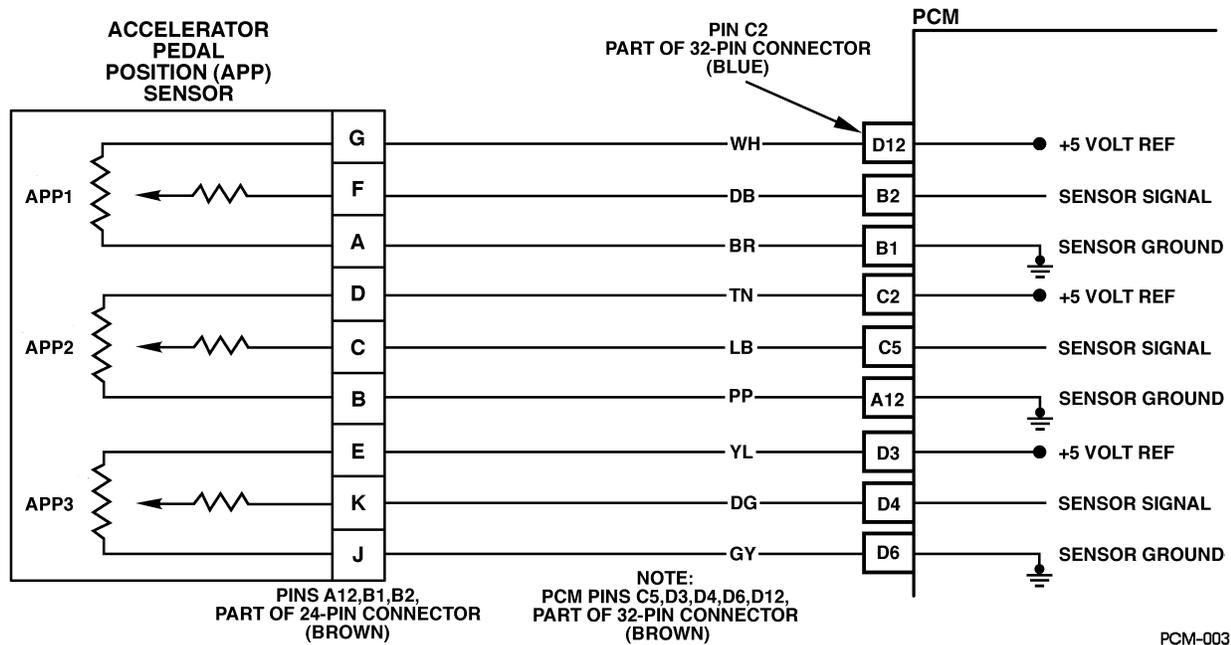
Figure PCM-17 Accelerator Pedal Position (APP) Sensor 2 Circuit High Voltage
