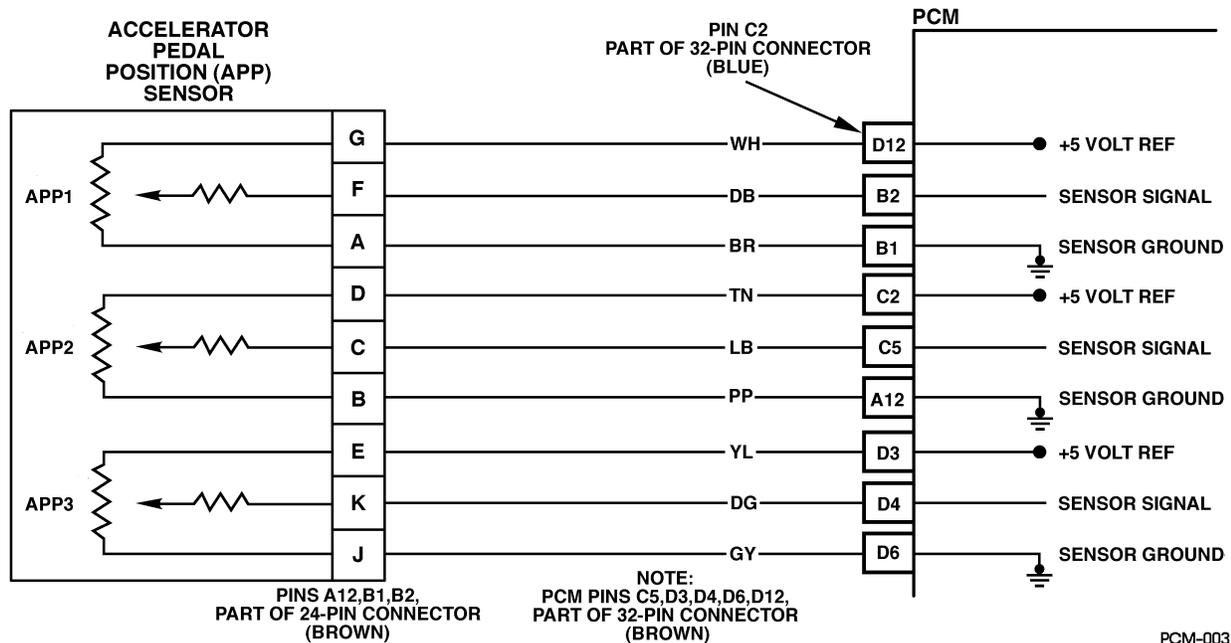
Figure PCM-21 Accelerator Pedal Position (APP) Sensor 3 Circuit High Voltage
