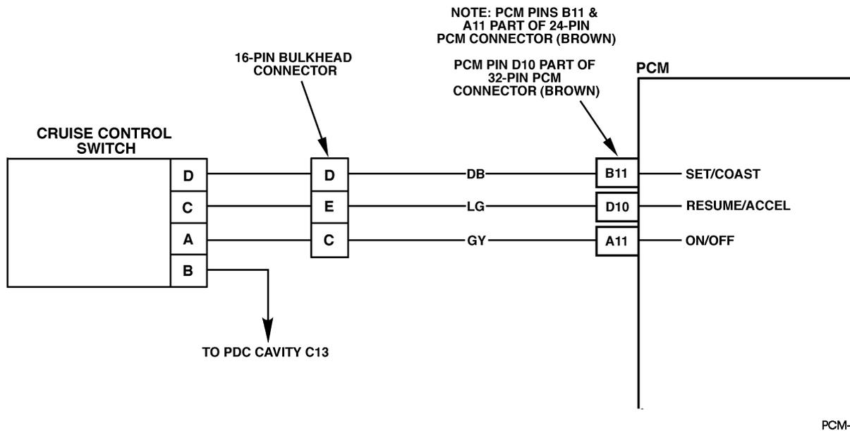
Figure PCM-33 Cruise Set Circuit
