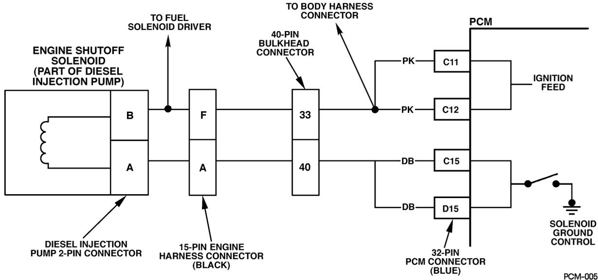
Figure PCM-11 Engine Shutoff Solenoid Control Circuit
