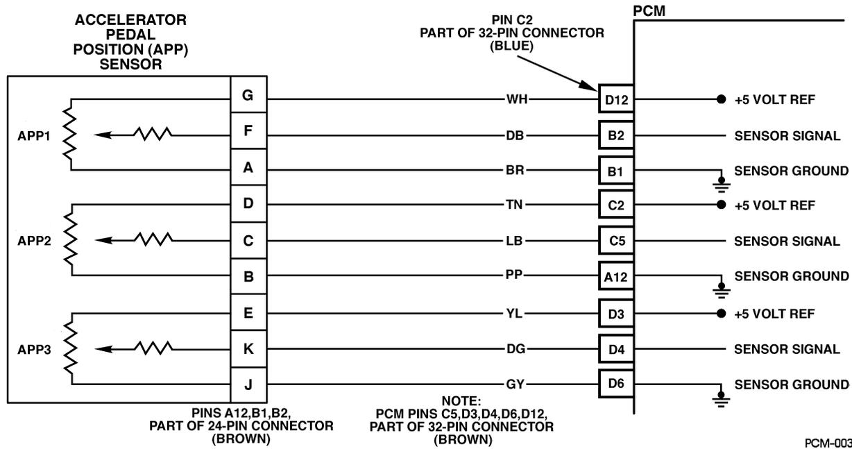
Figure PCM-16 Accelerator Pedal Position (APP) Sensor 2 Circuit Low Voltage
