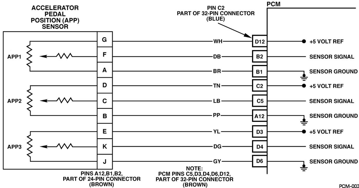
Figure PCM-7 Accelerator Pedal Position (APP) Sensor 1 Circuit Low Voltage
