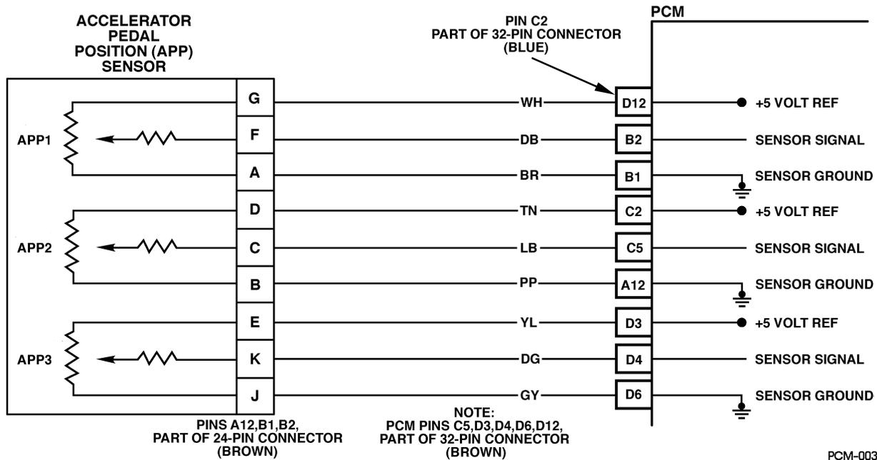
Figure PCM-6 Accelerator Pedal Position (APP) Sensor 1 Circuit Performance
