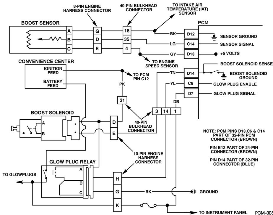
Figure PCM-44 Wastegate Solenoid Control Circuit
