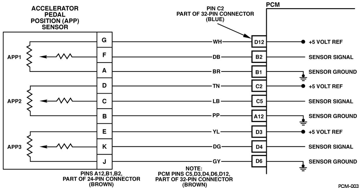
Figure PCM-18 Accelerator Pedal position (APP) Sensor 3 Circuit
