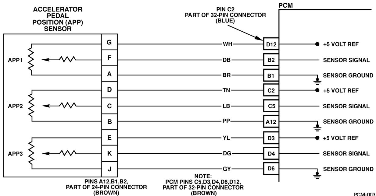
Figure PCM-19 Accelerator Pedal Position (APP) Sensor 3 Circuit Performance
