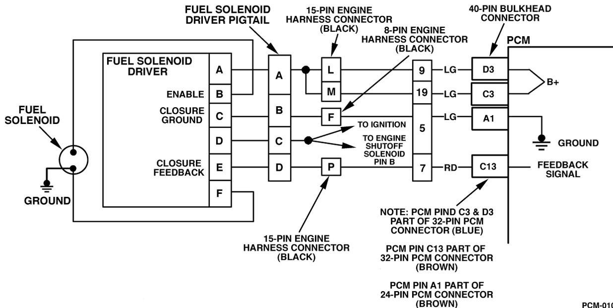
Figure PCM-37 Fuel Solenoid Response Time Too Short
