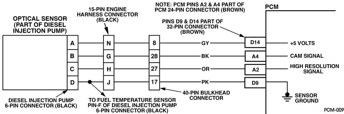
Figure PCM-26 Injection Pump Cam System
