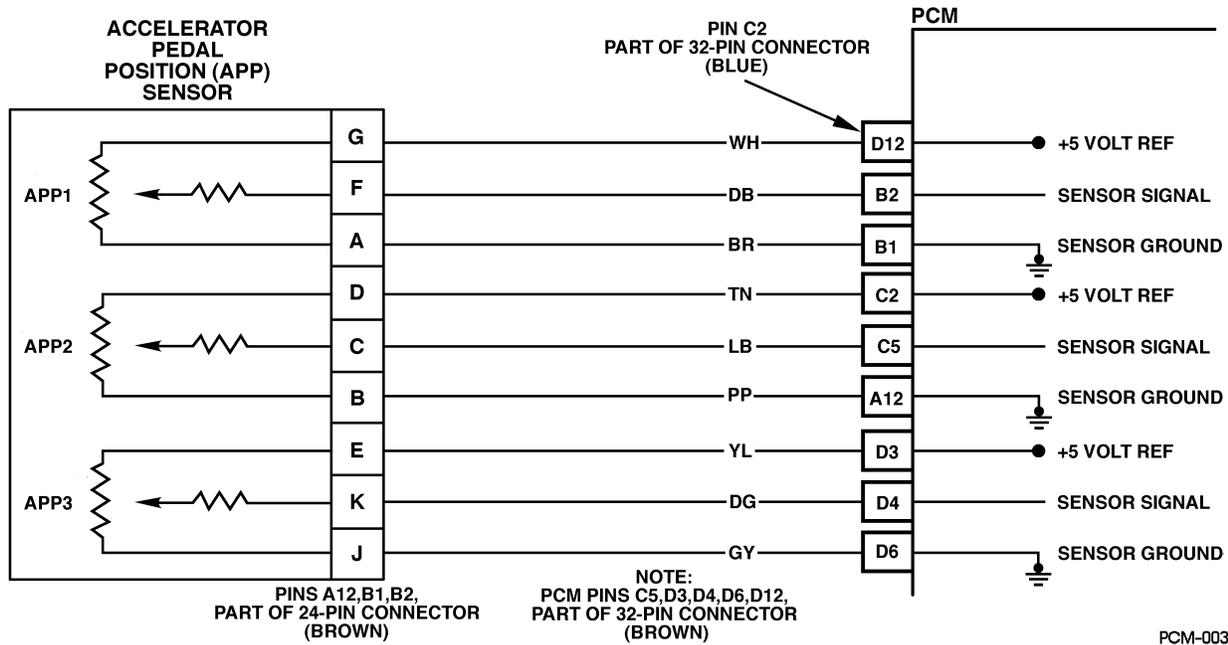
Figure PCM-8 Accelerator Pedal Position (APP) Sensor Circuit High Voltage
