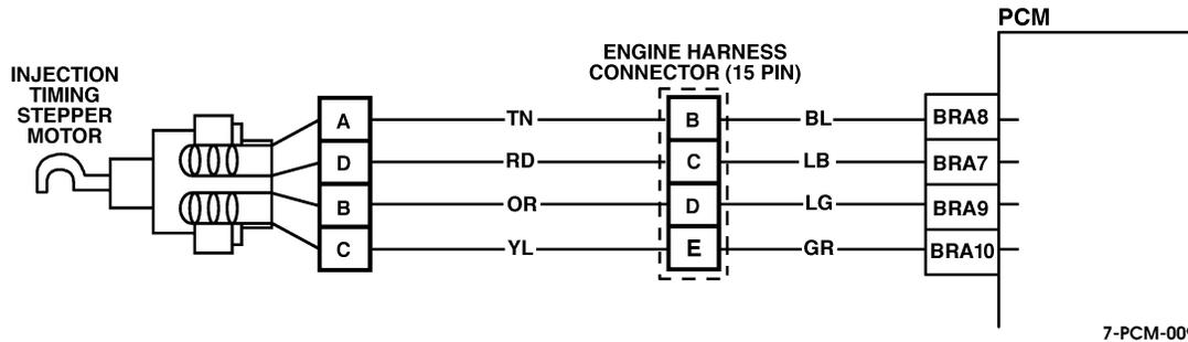
Figure PCM-36 Injection Pump Timing Offset Error
