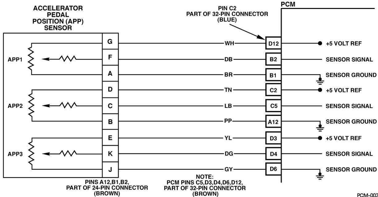
Figure PCM-20 Accelerator Pedal Position (APP) Sensor 3 Circuit Low Voltage
