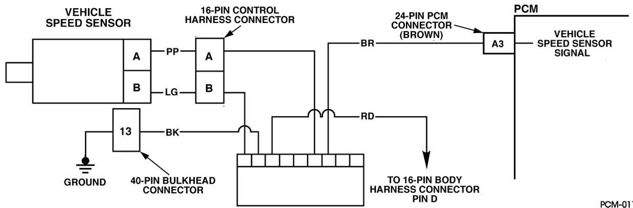
Figure PCM-31 Vehicle Speed Sensor Circuit
