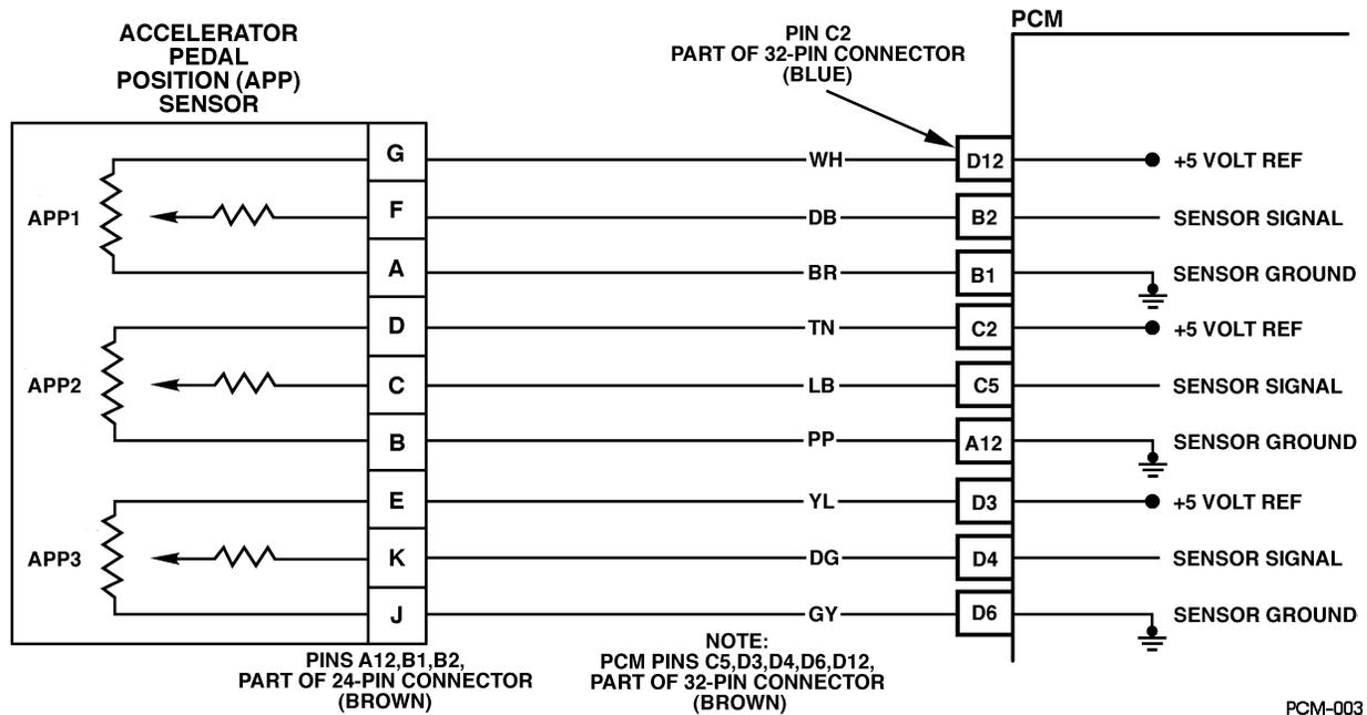
Figure PCM-35 Accelerator Pedal Position (APP) System
