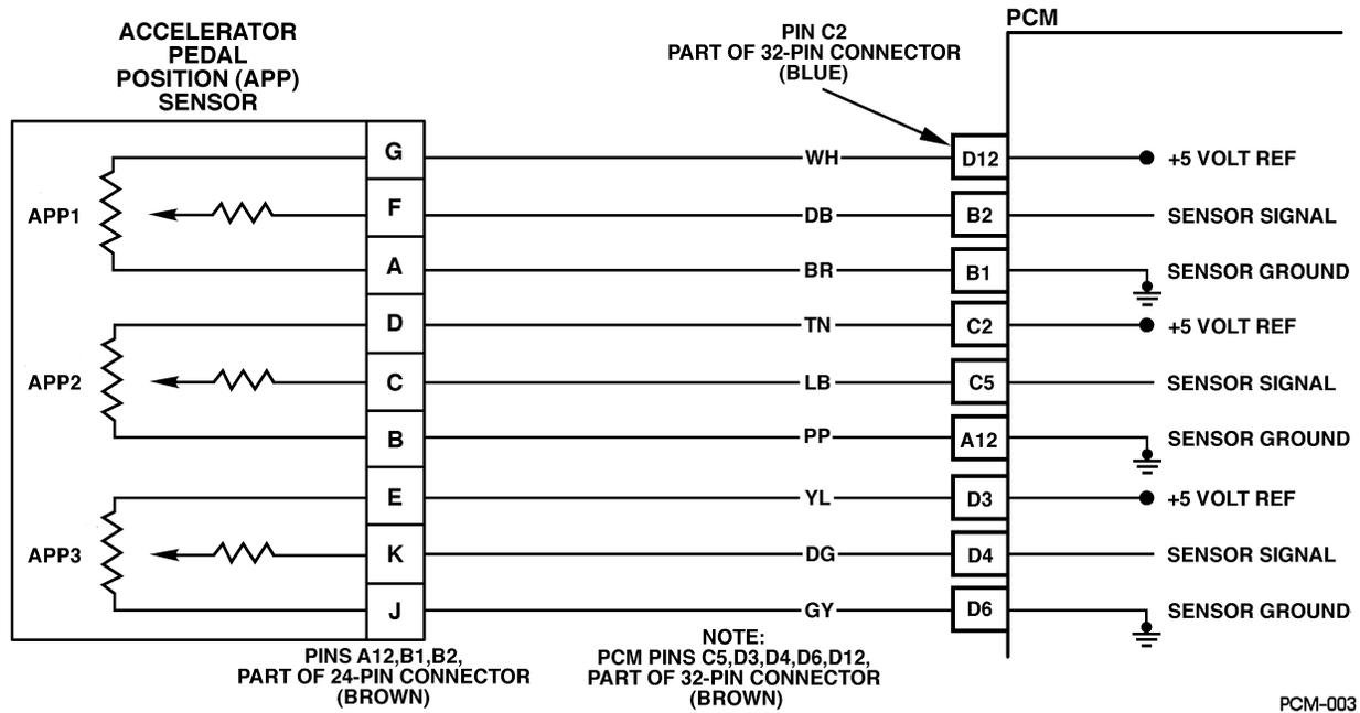
Figure PCM-14 Accelerator Pedal Position (APP) Sensor 2 Circuit
