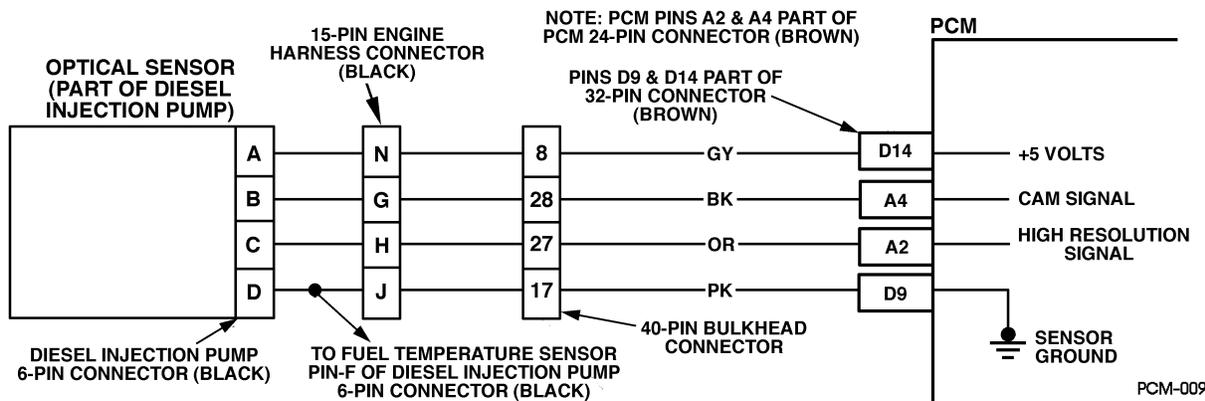
Figure PCM-28 Crankshaft Position (CKP) Sensor Circuit Performance
